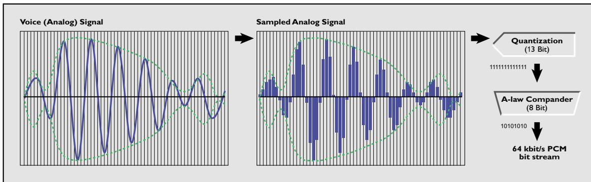
Figure 2 Converting a voice signal (Pulse Code Modulation, PCM)
