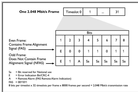
Figure 8 FAS framing format
