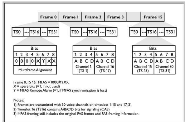
Figure 9 MFAS framing format
