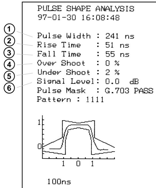
Figure 4 Example of pulse shape measurement screen
