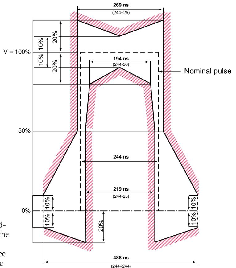
Figure 3 Mask of the pulse at 2.048 Mbps interface
