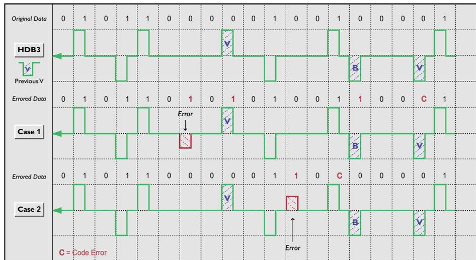
Figure 7 HDB3 error detection
