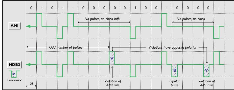
Figure 6 AMI and HDB3 line coding
