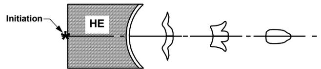
Figure 3. Stages in the development of an explosively formed projectile.
