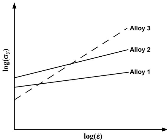
Figure 6. Strain rate sensitivity.
