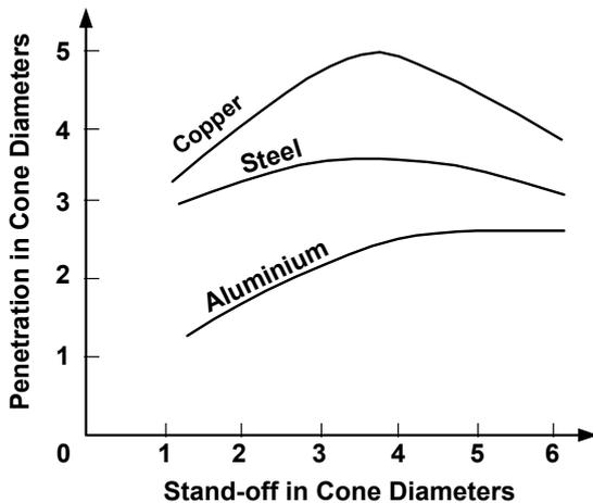
Figure 4. Penetration curves for various conical liners into a steel target.
