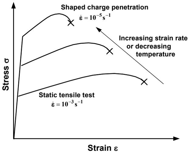
Figure 5. Tensile test curves at different strain rates.
