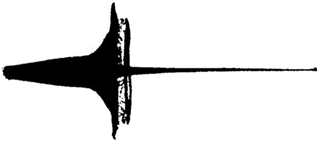
Figure 1. Flash X-ray of a collapsing copper cone.
