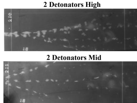
Figure 4. Conical shaped charge jet flash x-rays.
