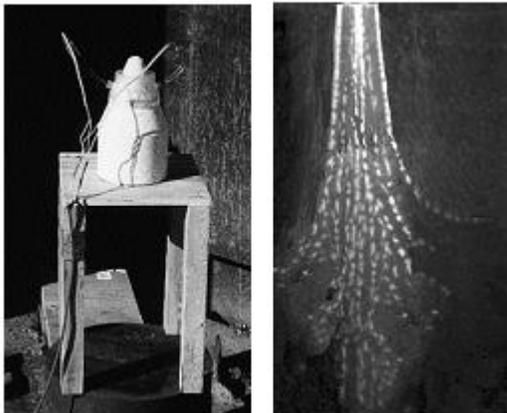
Figure 11. Selectable mode warhead test stand (left). X-ray of case 1 fan jet at 80 microseconds (right).
