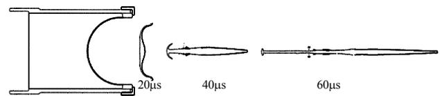
Figure 5. CALE model of a baseline hemispherical shaped charge.
