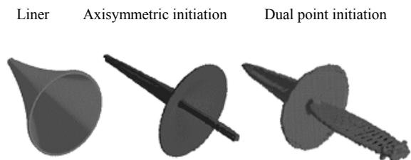
Figure 9. Comparison of CTH predicted standard jet vs. dual point initiated fan jet.
