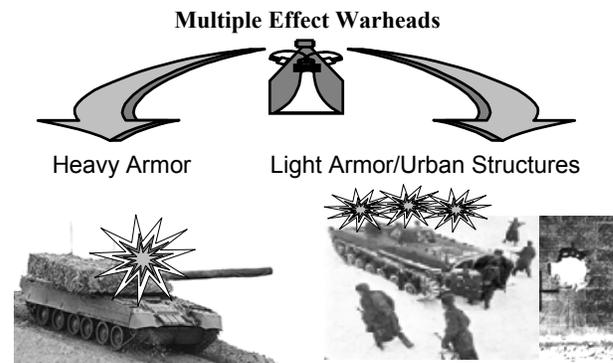
Figure 1. Selectable-initiation warhead against multiple targets.
