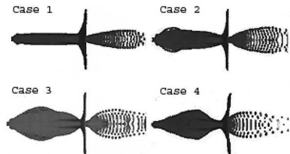
Figure 10. Jet profile as a function of detonator location at 35 microseconds.
