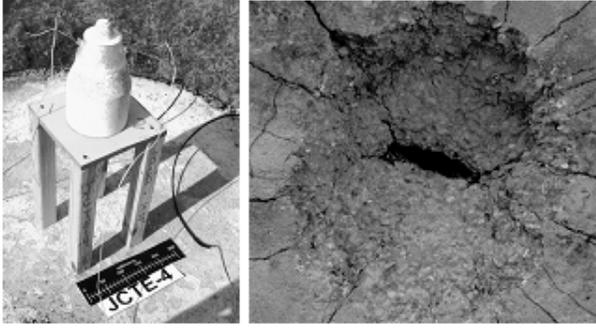
Figure 14. Dual initiation shaped charge concrete experimental setup and concrete target face.
