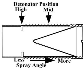
Figure 2. Conical shaped charge cross section showing two detonator locations.
