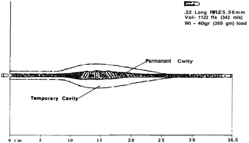
**FIWRL 5.-22 Lung RtJkz This solid lead round-nosed bullet yaws through 90° and travels base-forward for the last half of its tissue path.**
