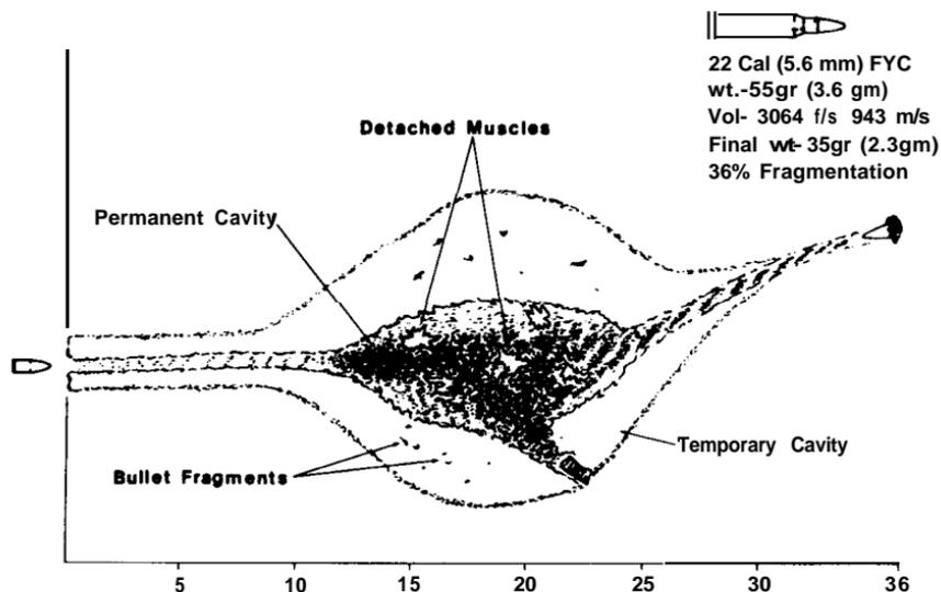
Figure 12.-22 metal-cased (M-16 rifle cased M-193 bullet). **This is the standard weapon of the U.S. Armed Forces, although it is soon to be replaced by a new rifle using the same caliber and cartridge but with a longer and slightly heavier (62 grain) bullet.**
