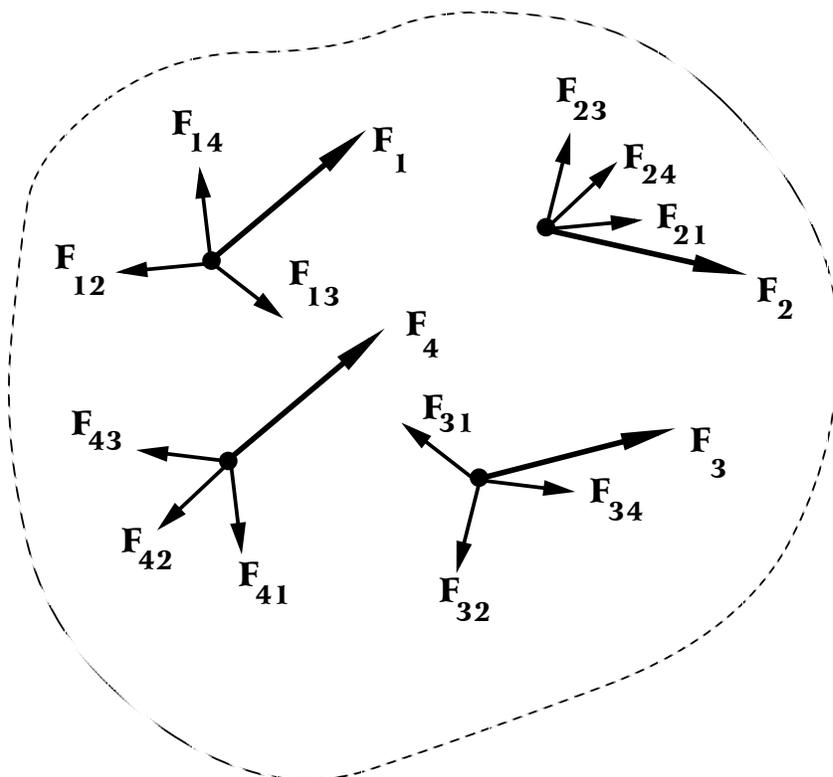
**Figure 1** A system of particles with internal and external forces.
