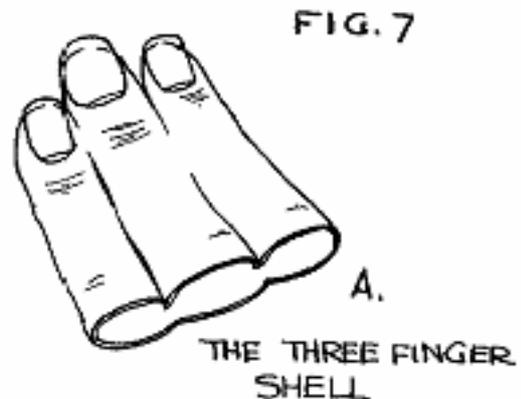
The improvement consists of a metal shape, or shell, made to slip over the first three fingers of the right hand, and cover as far as the second joints. (See Fig. 7A). (Some might prefer the last three fingers.)
