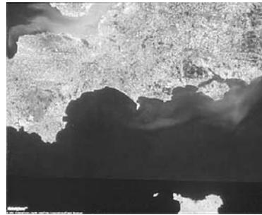
Three views of the British coastline. The Bill of Portland, barely visible in the first image, shows up as a small peninsula in the second and in detail in the third. Measurements based on each would produce different results for the coastline's length, and yet all three accurately represent the same coastline (GlobeExplorer).
