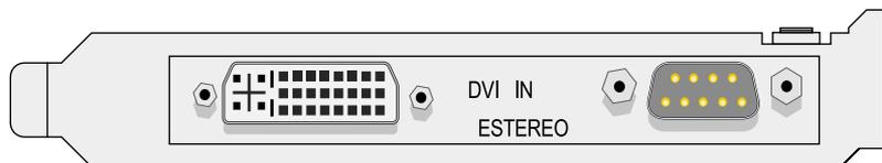
**Figure 1-1** SGC PCI-X Card Bulkhead View
