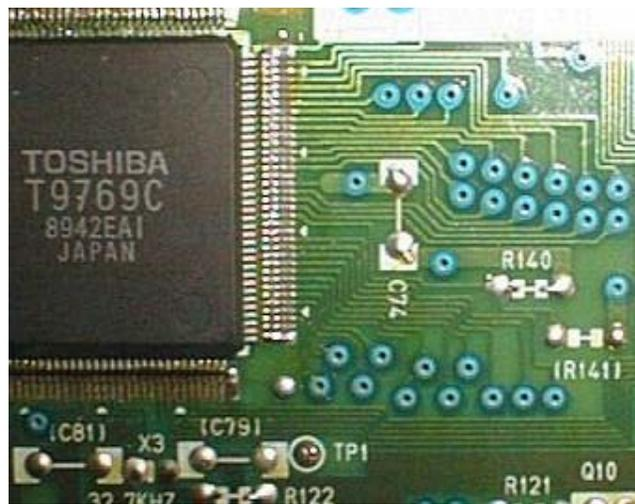
R140 and R141 on the back side of Panasonic FS A1WSX PCB
