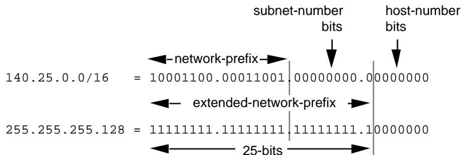
Figure 14: Example #2 - Defining the Subnet Mask/Extended-Prefix Length
