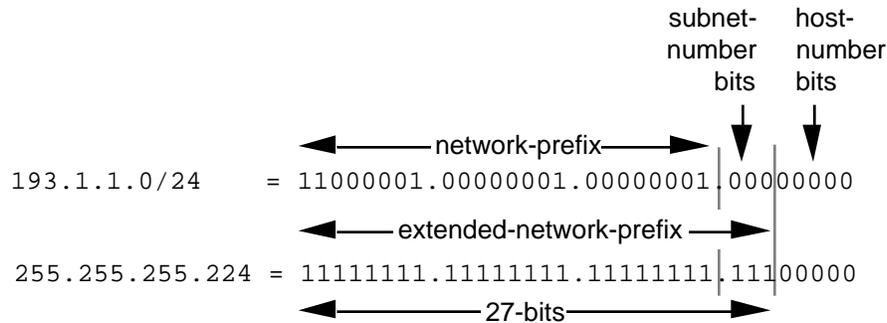
**Figure 11: Example #1 - Defining the Subnet Mask/Extended-Prefix Length**
