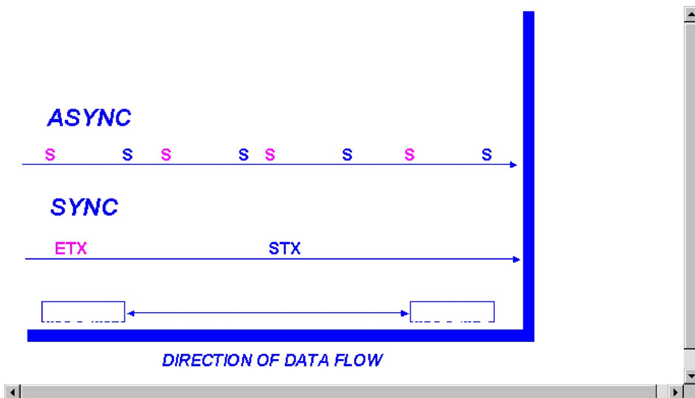
In asynchronous transmission, data is transmitted one character at a time. Each character is bracketed by a start bit and one or more stop bits. Asynchronous transmission is also called *start-stop* transmission. The asynchronous characters are not evenly spaced along the transmission medium. In gaps between characters, the line is idle; nothing is transmitted. The characters are transmitted independently with regard to timing signals.
