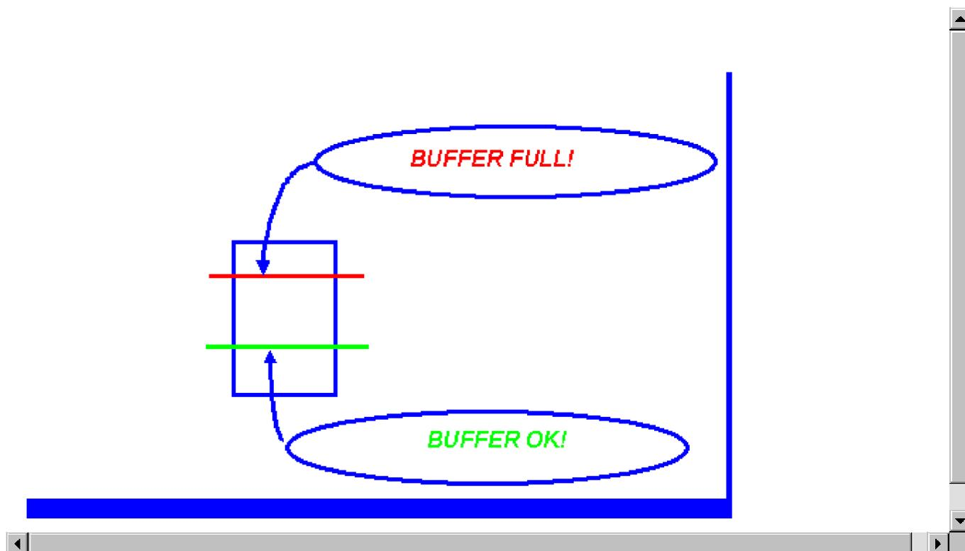
One of the ways that computers and modems take care of differences between data transfer rates is through the use of buffers. Both the communication application on the DTE side and the modem on the DCE side can use buffers as a temporary storage location for data. However, problems can still occur even with buffers in place.
