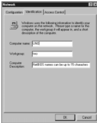
Figure 9.1 NetBIOS names can be set up to 15 characters in Microsoft computers. The name of this Windows 95 computer is "UNO."
