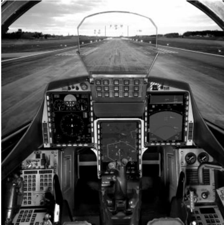
**Figure 1.2:** On the left is the flight data display, on the middle the horizontal situation display, on the right the multi-sensor display, and straight ahead is the head-up display.
