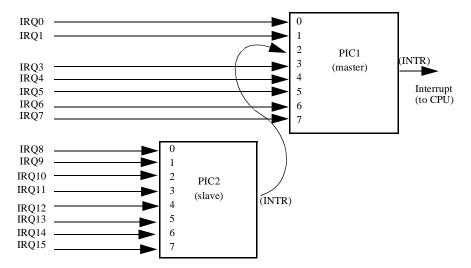
Figure 3. PIC1 (master) and PIC2 (slave) Interconnection
