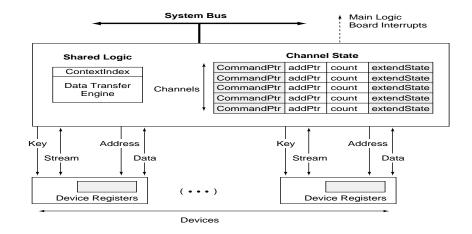
Figure 9. DBDMA controller model
