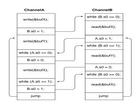
Figure 11. Synchronizing flow-controlled channel programs
