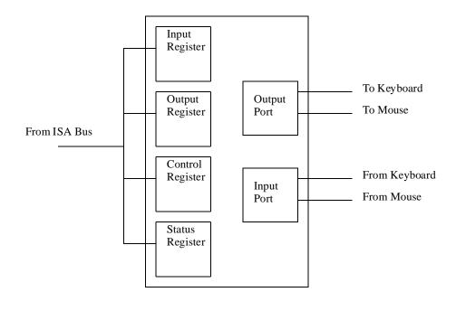
Figure 4. Block Diagram of Keyboard/Mouse Controller Register
