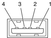
The iMac provides 5-volt power to the USB ports. The maximum current available is 500 mA on each port (1 A total).
