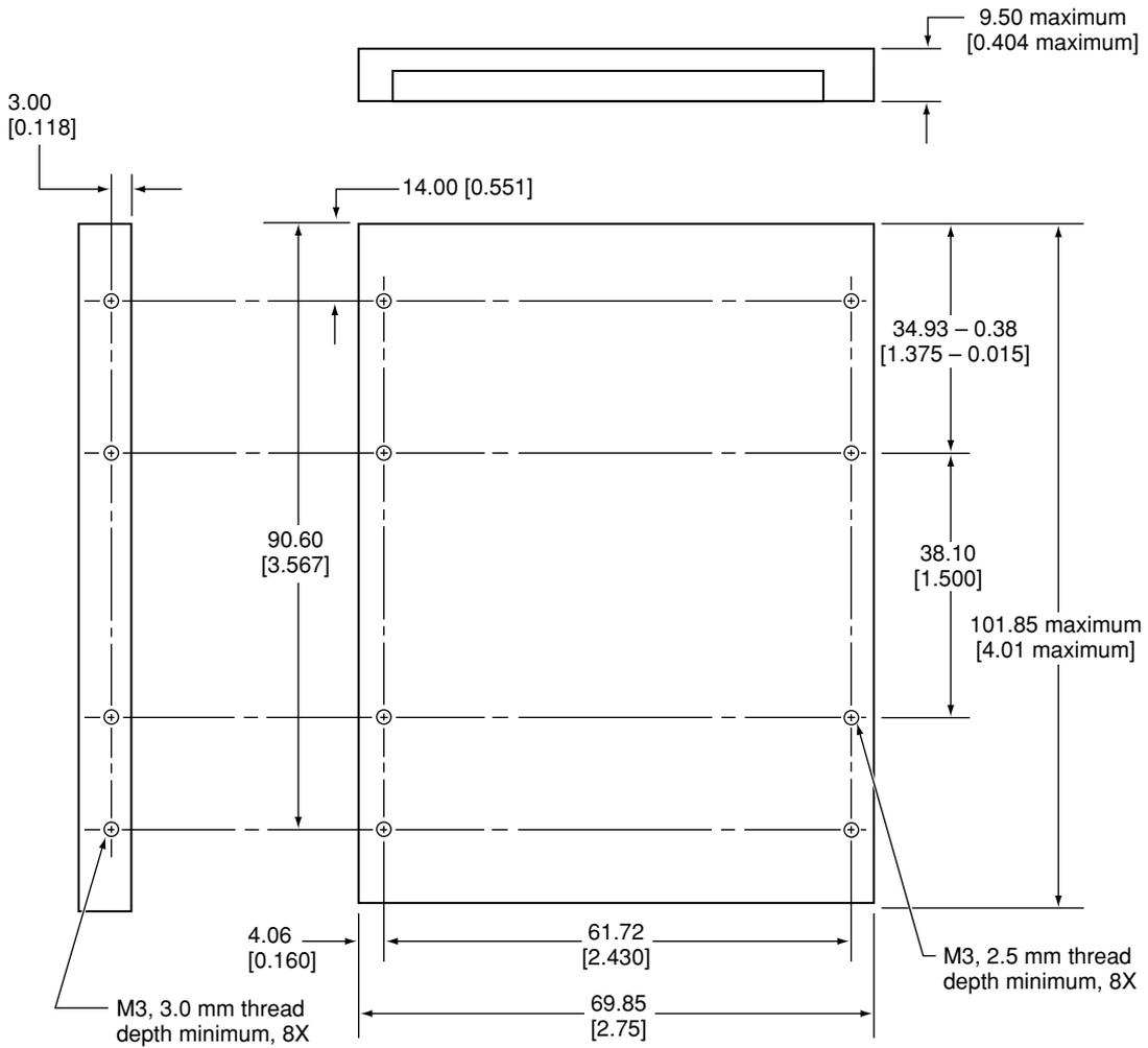
Note: Dimensions are in millimeters [inches].
