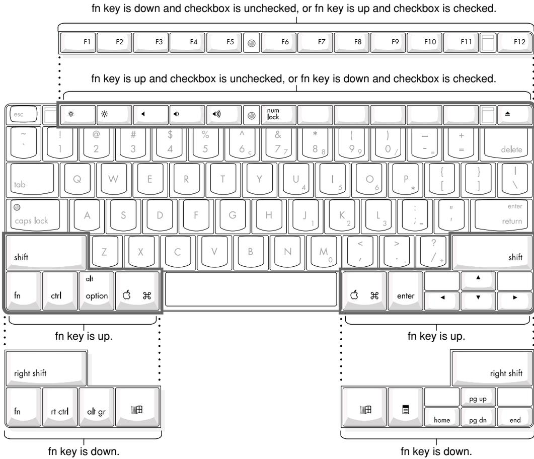
**Figure 3-7** Embedded numeric keypad operation
