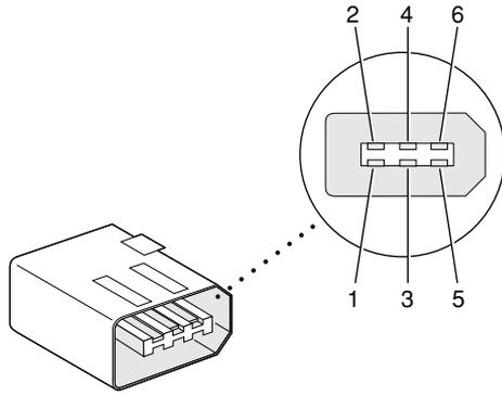
**Table 3-2** Pin assignments on the FireWire connector
