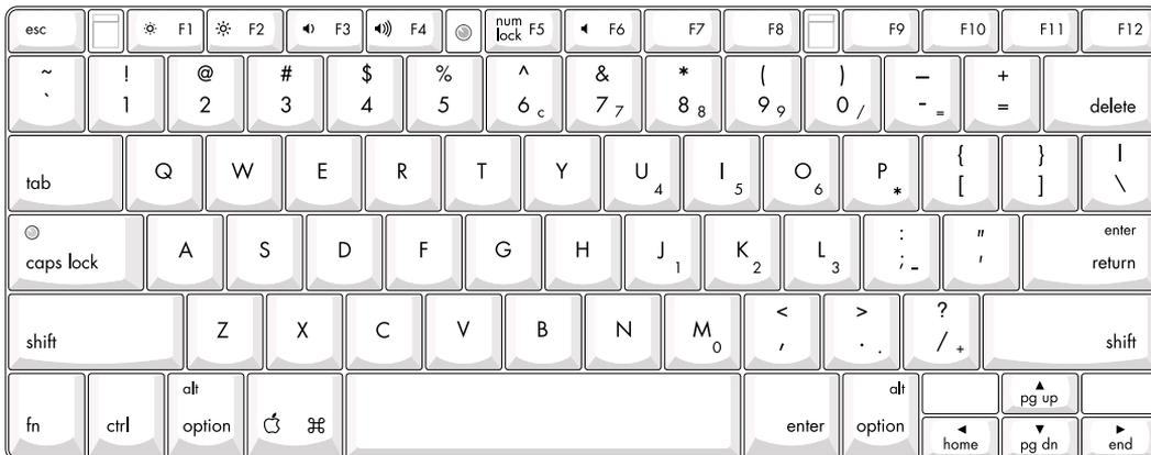
**Figure 3-6** Embedded numeric keypad operation
