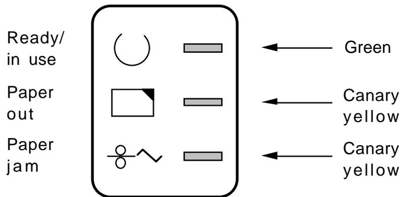
Different combinations of lights indicate the different states of operation, as shown in Table 1-2. The lights are also used as an indication of machine malfunctions, which are described in Table 1-3.
