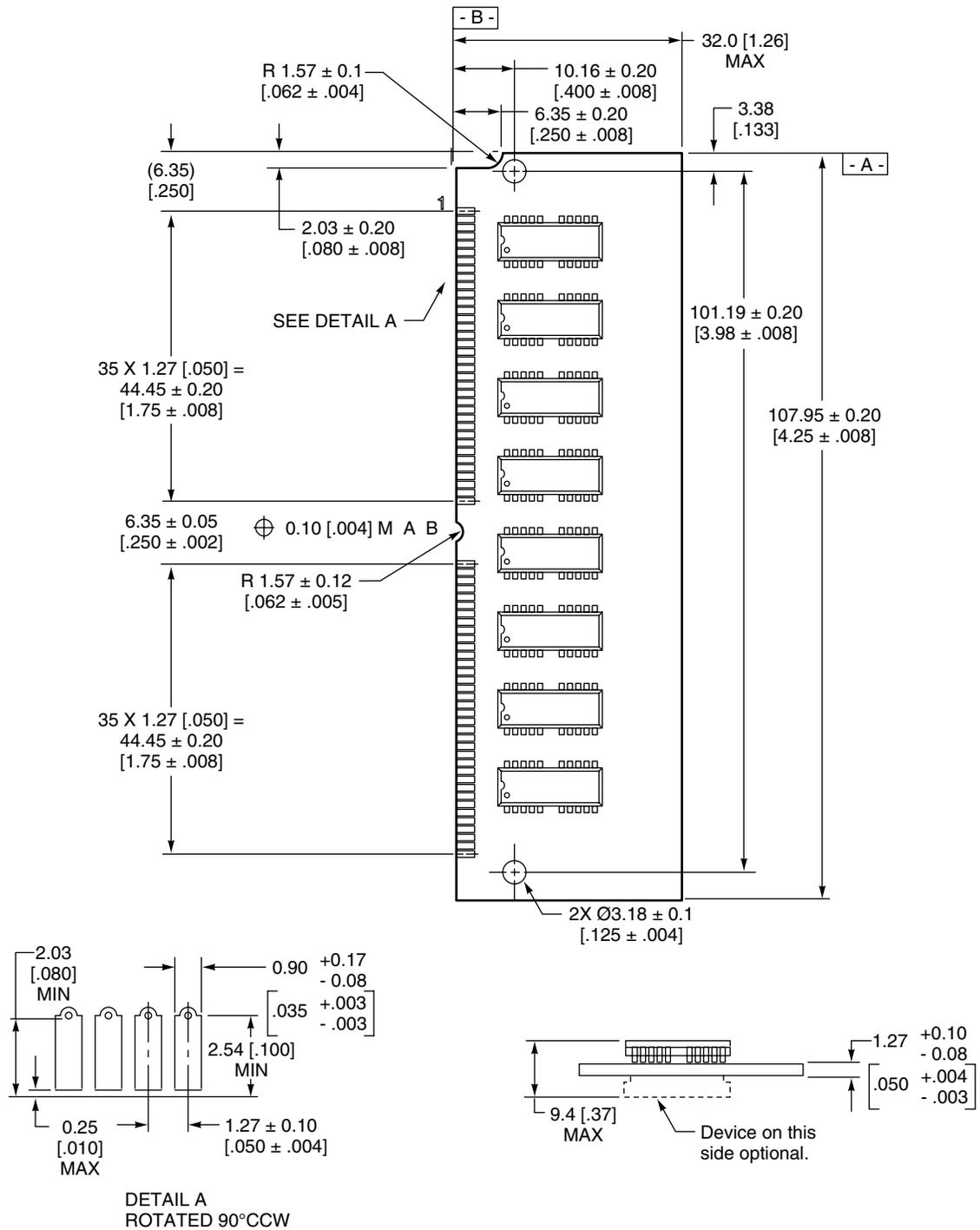
Note: Dimensions are in millimeters with inches in brackets.
