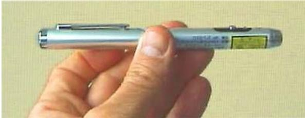
Inexpensive laser pointer (1 mw, 650 nm red)
