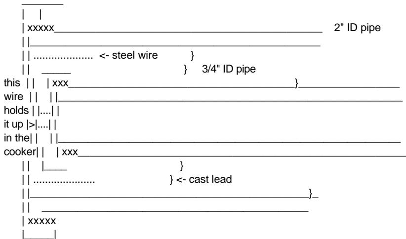
We dug into the side of a sand pile and built a chimney out of firebrick. Then we stood the assembled pipe and wire on end in the chimney, sitting on some bricks. We then had a blowtorch heating up the chimney, so that the pipe was red hot. Then we poured molten lead into the space between the pipes. If the caps aren't screwed on real tight, some of the lead will leak out. If that happens, turn off the blowtorch and the pipe will cool enough and the lead will stiffen and stop the leak.
