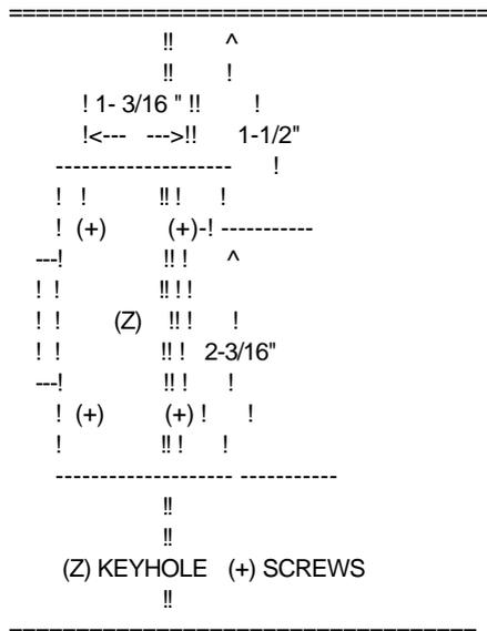
AFTER THIS IS ACCOMPLISHED, THE LOCK CAN BE PUSHED BACKWARDS DISENGAGING THE LOCK FROM THE COVER PLATE. THE FOUR BOLTS OF THE COVER PLATE CAN THEN BE RETRACTED BY TURNING THE BOLTWORKS WITH A SIMPLE KEY IN THE SHAPE OF THE HOLE ON THE COIN PLATE (SEE DIAGRAM BELOW). OF COURSE, THERE ARE OTHER METHODS AND DRILLING PATTERNS.
