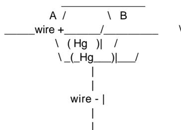
When the drop of mercury ("Hg" is mercury's atomic symbol) touches both contacts, current flows through the switch. If this particular switch was in its present position, A---B, current would be flowing, since the mercury can touch both contacts in the horizontal position.
