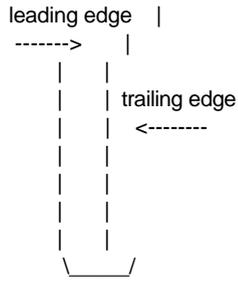
The leading edge and trailing edge should be sanded with sandpaper so that they are rounded. This will help make the rocket fly straight. A two inch long section of a plastic straw can be attached to the rocket to launch it from. A clothes hanger can be cut and made into a launch rod. The segment of a plastic straw should be glued to the rocket engine adjacent to one of the fins of the rocket. A front view of a completed rocket bomb is shown below.
