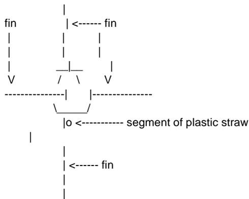
By cutting a coat hanger at the indicated arrows, and bending it, a launch rod can be made. After a fuse is inserted in the engine, the rocket is simply slid down the launch rod, which is put through the segment of plastic straw. The rocket should slide easily along a coathanger, such as the one illustrated on the following page:
