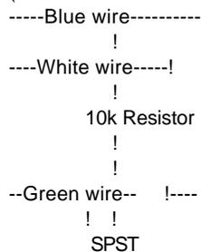
What this does in effect is keep the hookswitch / dial pulse switch (F to RR loop) open while holding the line high with the resistor. This gives the same voltage effect as if the fone was 'on-hook', while the 10k ohms holds the voltage right above the 'off hook' threshold (around 22 volts or so, as compared to 15-17 or normal off hook 48 volts for normal 'on-hook'), giving Test Set Version 2.
