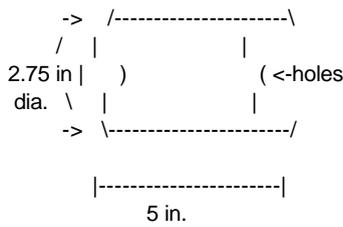
2) Drill four rows of holes in pipe nipple. Use table 1 for diameter and location of holes.
