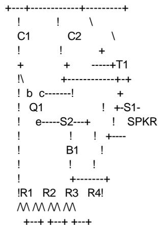
Now that you are probably thoroughly confused, let me explain a few minor details. The potentiometer area is rigged so that the left pole is connected to the center pole of the potentiometer next to it. The middle terminal of T1 is connected to the piece of wire that runs down to the end of the battery.
