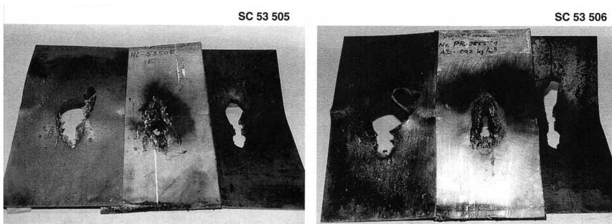
**Figure 4.** Slits and craters in the 2 mm mild steel plate on the left side, the 20 mm Dyneema plate in the middle and the slit in the 4 mm mild steel plate on the right side.
