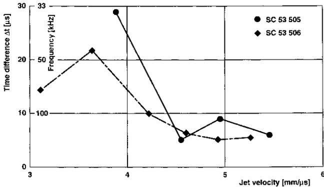
**Figure 5.** Time differences  $\Delta t$  of the disturbances of the passing jet as a function of the jet velocity.
