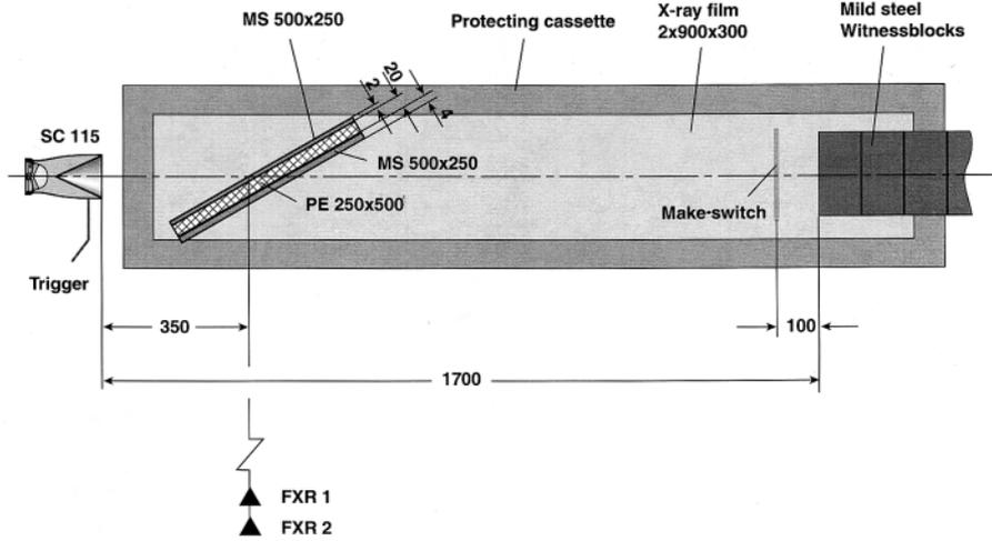
Figure 1. Test setup of bulging armour against 115 mm shaped charge in front of double flash X-ray diagnostic; all distances in mm.
