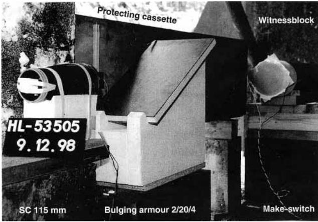
Figure 2. Picture of the test setup with the shaped charge in front of a bulging armour 2/20/4 of mild steel plates on 20 mm Dyneema under 60°, the make-switch on the right side with the witness blocks for measuring of residual penetration. In the background the protecting cassette for the 1.8 m long FXR films.
