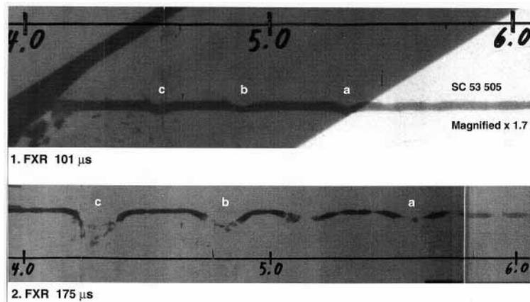
**Figure 6.** Comparison of the disturbances of the jet on the flash X-ray exposures after 101 μs and 175 μs which means shorter time after the interference with the bulging plate and later times of firings SC 53505. The earlier picture is 1.7 times magnified to the later picture for better comparison.
