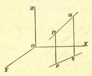
Let PQ be the straight line, pq its projection on the plane XOY by lines parallel to OZ. Then the co-ordinates x and y of any point in PQ are the same as the co-ordinates x and y of its projection in pq.
