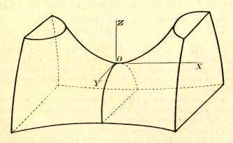
The surface is on both sides of the plane z=0, and extends to an infinite distance in both directions.
