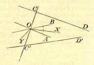
Let O be the middle point of CC', the shortest distance between the two straight lines CD, C'D'. Through O draw OA, OB parallel to CD, C'D', and let OX, OY bisect the angle AOB. Take OX, OY, OC for axes of co-ordinates; then, if AOB be  $2\alpha$ , the equations of OA, OB are  $y = x \tan \alpha z = 0$ , and  $y = -x \tan \alpha, z = 0$ .
