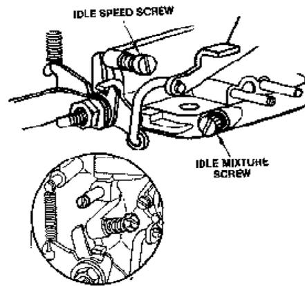
It is important to follow all linkage and lever installation instructions. The number one and two reasons for tuning errors are improper linkage installations and over tightened linkage nut, causing a binding in linkage assembly.
